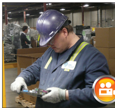
Worker in new Sims CRT recycling plant strips out printed circuit boards. Behind him in the warehouse are hundreds of skids with CRT waste.
